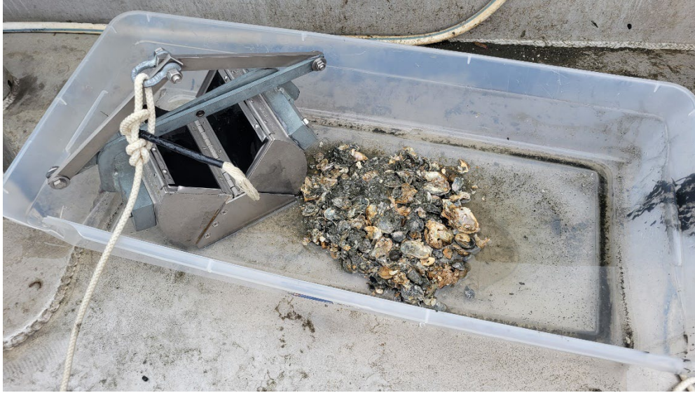
Figure J.2. A Wildco® Petit Ponar® (6'' x 6'', 24 lbs, sample volume = 2,400 mL) was deployed at each location to sample benthic habitat. Example of a ponar grab of loose shells, shell hash, and sand.
